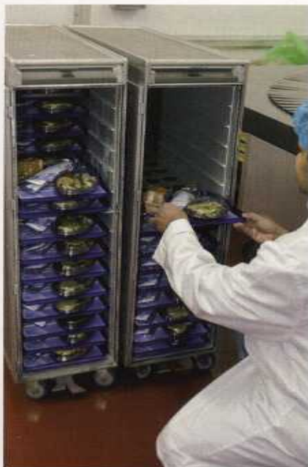
Once the trays have been prepared, they are loaded into trolleys. The trolleys each hold 28 meals and are the standard configuration used by most of the world's airlines.
