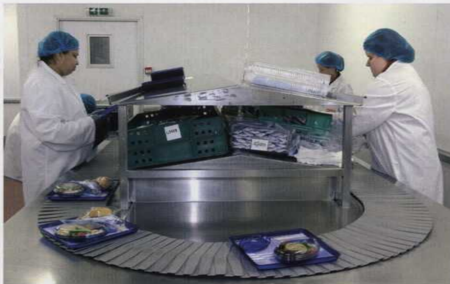
As up to 300 identical meals need to be provided to some customer airlines, FFL has found that the most efficient method is to make use of a circular carousel for loading each meal tray. Each member of staff is responsible for loading an individual course on every tray.
