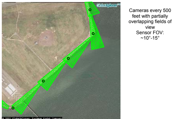
Figure 17 – Recommended Perimeter Configuration
